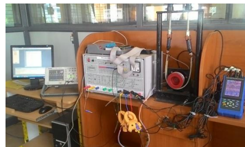
Fig. 5 Overall Experimental Setup in Real Time with DSPIC30F4011
